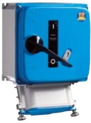
TUNNEL54 SERIES Interlocked high power socket-outlets for tunnel fans IP66 > IK10 400°C for 120'
