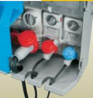
Clamping the plug cables is no longer time-consuming; simply place the cable into the conical groove in order to automatically prevent tugging ensuring safety.
